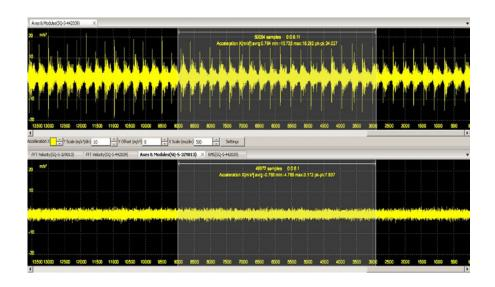
FFT Analysis of 2 accelerometers synchronous channel
